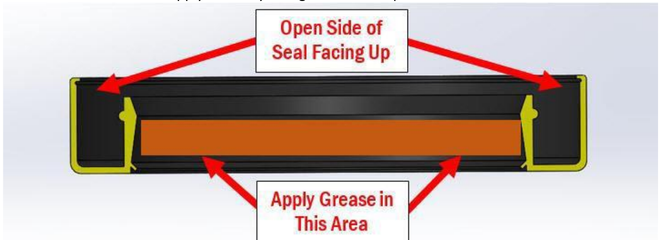
Figure 35: Seal Orientation and Grease Location
