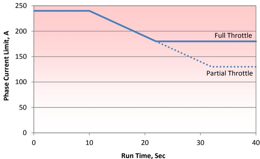
Figure 9: Current limit behavior for "burst" settings.
