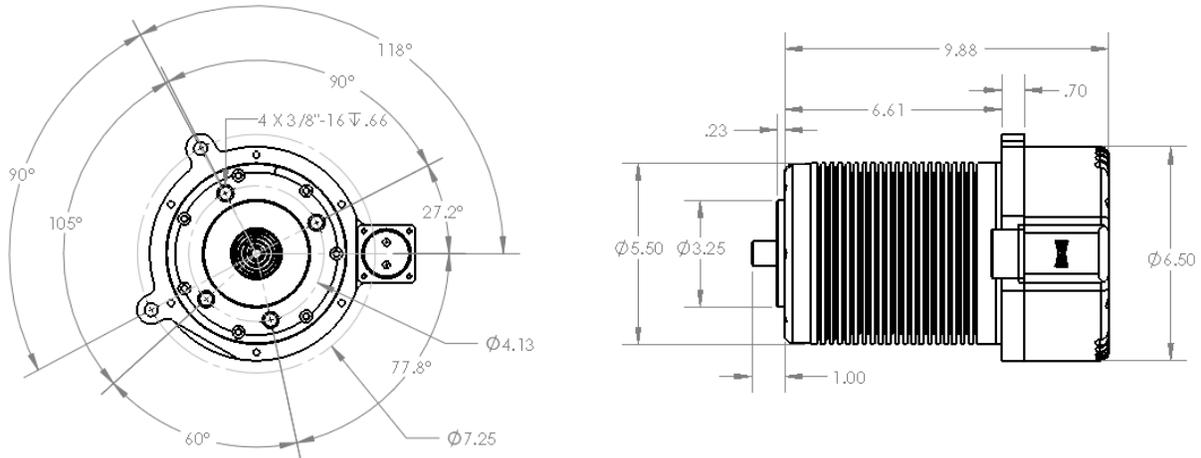
Figure 2: Motor mounting dimensions
