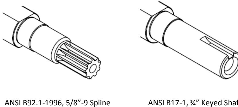
Figure 1: Standard Shaft Connections
