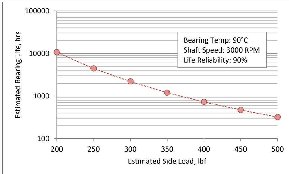
Figure 3: Front bearing estimated life vs radial load.
