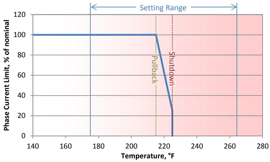
Figure 10: Phase current limit derating with temperature.
